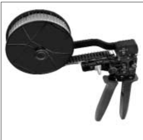
Hand crimp tool with spool The hand crimping tool feeds the contact on a tape and the contacts are separated automatically during the crimping process. Contacts are moved forward by hand operation.
